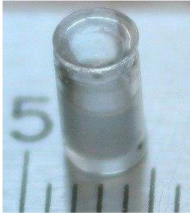
Pic.2. Photo of microfabricated atomic cell. Cell length - 6 mm; diameter - 4 mm.
